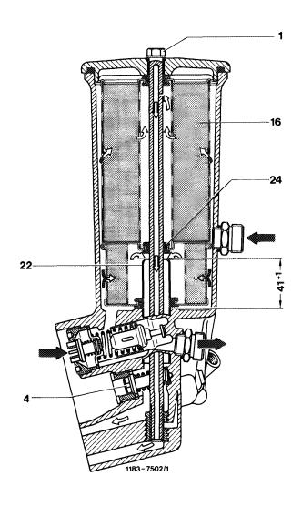
Check pressing-in depth of riser pipe in oil filter. Height of riser pipe from upper edge of pipe up to contact surface of filter element should not exceed 41 + 1 mm. If the height exceeds 42 mm, renew complete oil filter.
