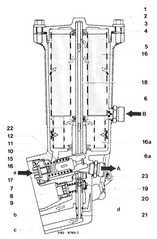
Coming from feed duct (a), the oil flows through return flow locking valve (16 and 17) into oil filter housing and flows directly to combiantion filter element.
