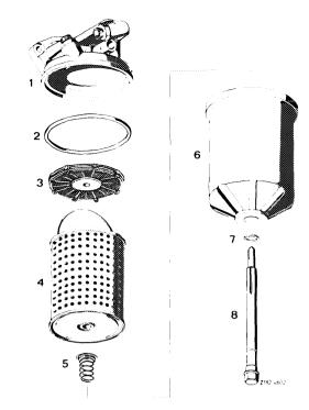
Clean main flow filter plate element with holding pliers 110 589 00 68 00 in benzine.
