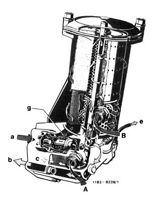
If the filter element is badly contaminated and the differential pressure between the dirty and the clean side of the filter exceeds 3.5 bar, the bypass valve (8 and 9) opens. The oil will then flow to engine in uncleaned condition.
