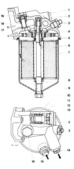
When the filter element is badly contaminated and the differential pressure between the dirty and the clean side of the filter exceeds 3.5 bar gauge pressure, the bypass valve (17) will open. The oil will then flow to engine in uncleaned condition.
